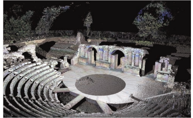
Laser scanner image of the Theatre at Butrint.
