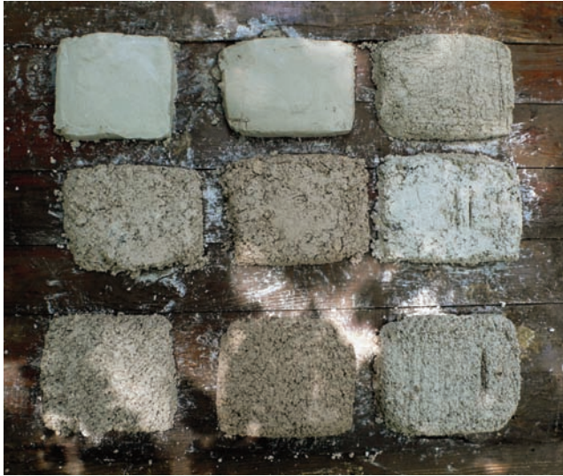
Examples of different grades of mortar used to instruct conservation trainees in mixing period replica mortars.
