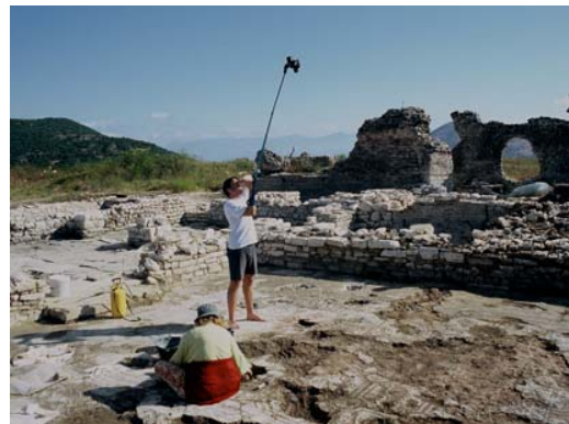
Fig. 29. Photogrammetric imaging of church mosaic under conservation.
